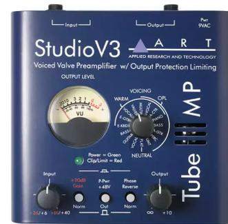
The Tube MP Studio V3 delivers warmth and fatness to any audio source while maintaining an exceptionally low-noise signal path. While its primary function is as a microphone preamp with +48V phantom power, variable gain and phase reverse switching, the Tube MP is also an exceptionally versatile tube driven direct box for any instrument source.
