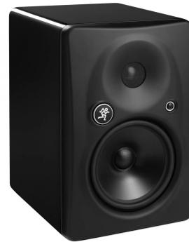
The cast-aluminum Zero Edge Baffle keeps diffraction to a minimum for excellent imaging, while the optimized waveguide provides a wide sweet spot, and the integral cabinet damping eliminates midrange artifacts. The internally braced wood cabinet is OmniMount ready, allowing it to be mounted easily on a wall or ceiling.
